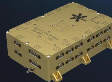
SpaceWire-router and on-board storage device of the on-board computer complex
