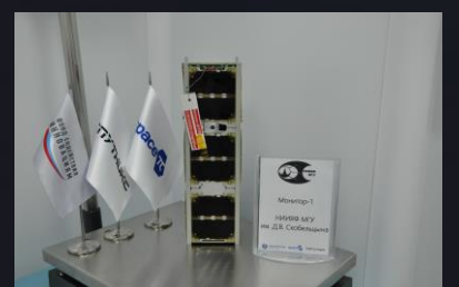
Monitor-1 NIYAF MSU Mass – 4 kg Purpose – Ed-Scientific sat Launch date – August 9, 2012
