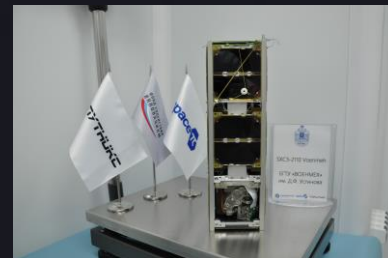
SXC3-2110 Voennmeh BSTU Voennmeh Mass – 4 kg Purpose – Ed-Scientific sat Launch date – August 9, 2012
