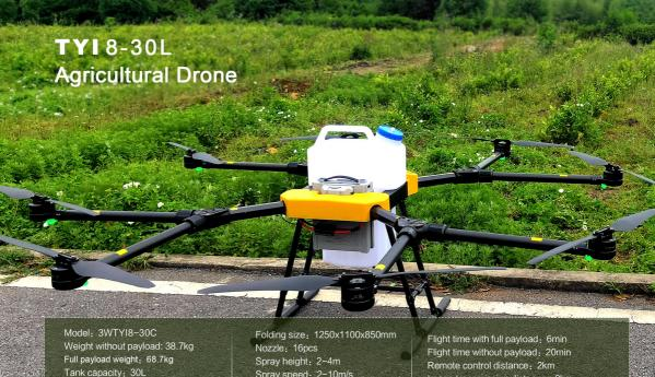
Axle distance: 2426mm Propeller diameter: 34inch Unfolding size: 3289x3289x850mm Spray speed: 2-10m/s Spray width: 6-8m Spray efficiency: 50ha/h Max flight speed: 15m/s
